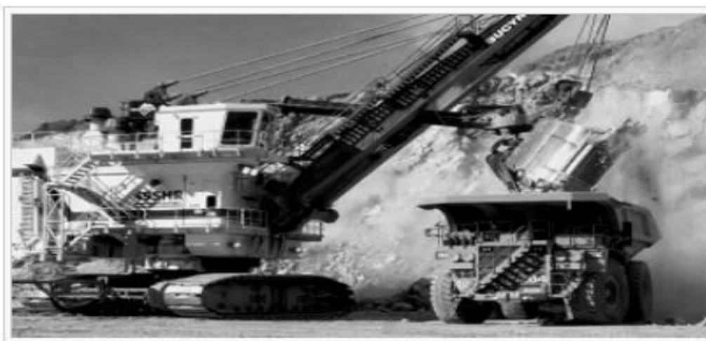
Figure 7.9: A Bucyrus rope shovel loading oil sands material into a Caterpillar truck. For an idea of the size of this shovel, the truck being loaded in this image is the same as the truck in above Figure.
