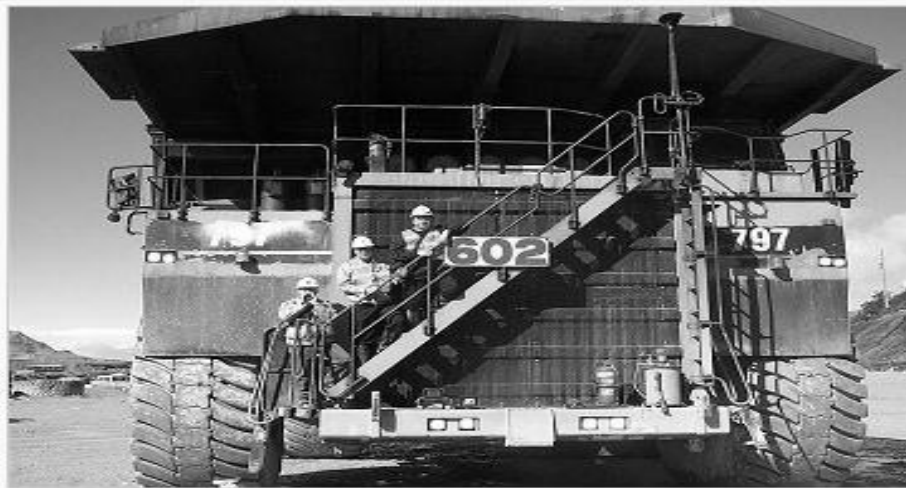
Figure 7.8: A Caterpillar 797 Truck Used in the Extraction of Oil Sands for Hauling the Extracted Sand
